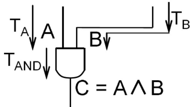
$$T_A < T_B \Rightarrow T_C = \begin{cases} T_A + T_{AND} & \text{if } A = 0 \\ T_B + T_{AND} & \text{if } A = 1 \end{cases}$$
