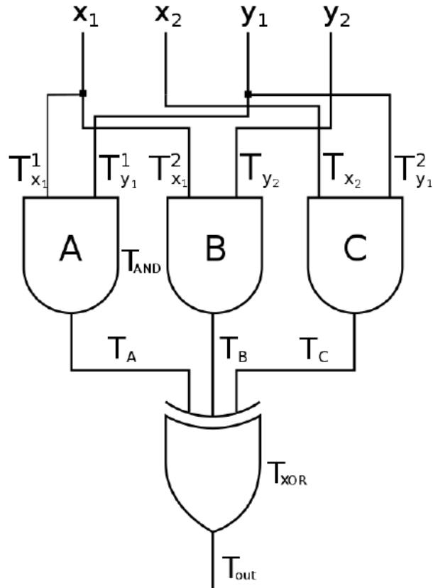
$$T_A = \begin{cases} T_{y_1}^1 + T_{AND} & (\text{if } y_1 = '0') \\ T_{x_1}^1 + T_{AND} & (\text{if } y_1 = '1') \end{cases}$$
